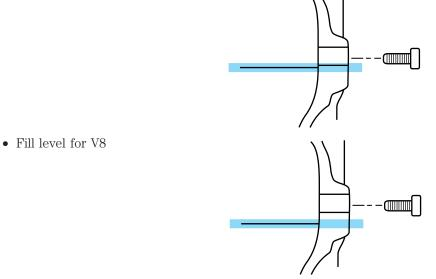
4. Add enough fluid through the filler opening to bring the fluid up to the recommended levels.
